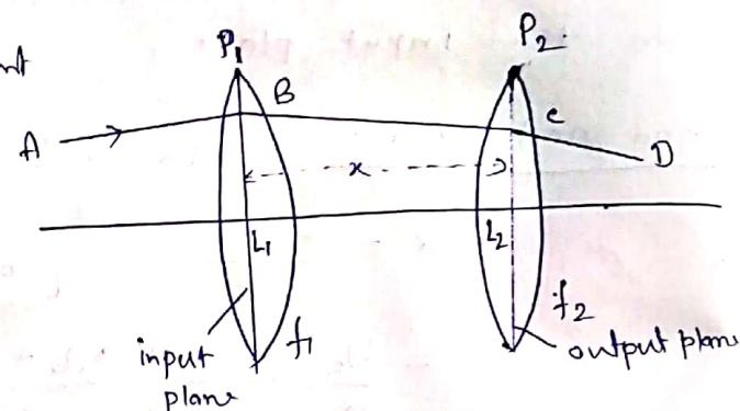
(i) Thin lens refraction at  $L_1$  represented by thin lens matrix,  $[S_{\text{thin}}]_1 = \begin{bmatrix} 1 & 0 \\ -\frac{1}{f_1} & 1 \end{bmatrix}$
