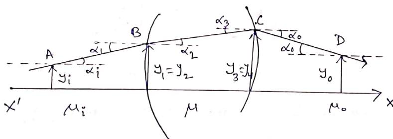
A ray of light AB travelling in a homogeneous medium of refractive index  $\mu_i$  meets the refracting surface at B. where it suffers refraction, travels along BC. in a medium of refractive index  $\mu$  and emerges as the ray CD into the medium of refractive index  $\mu_0$  after refraction at C.
