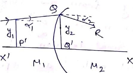
Output ray makes an angle  $\alpha_2$  with the axis. The distance  $y_2$  of the point  $Q$  from the axis is the same for the input ray as well as the output ray. Therefore,  $(y_2, \alpha_1)$  are the co-ordinates of the point  $Q$  from for the input ray and  $(y_2, \alpha_2)$  for the output ray.
